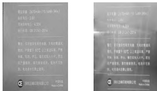
a) 空白样 a) Blank sample b) 附着力测定后 b) After testing adhesion
